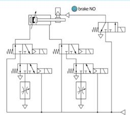
This circuit example permits the selection of different speeds (rapid or inching) for either forward or reverse motion. The brake is activated by a 3/2 solenoid valve.
