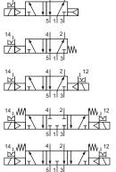
M-04-510-HN-xxx 5/2-way, single solenoid, air spring return M-04-511-HN-xxx 5/2-way, single solenoid, mechanical spring return
