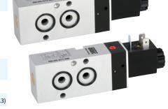
Electrically operated spool valve. The manual override is detent and is operated by screw driver. The model KN-55 has a coil with enhanced humitidy resistance and a additional gasket at the coil. The location pin, screws and seals are included.
